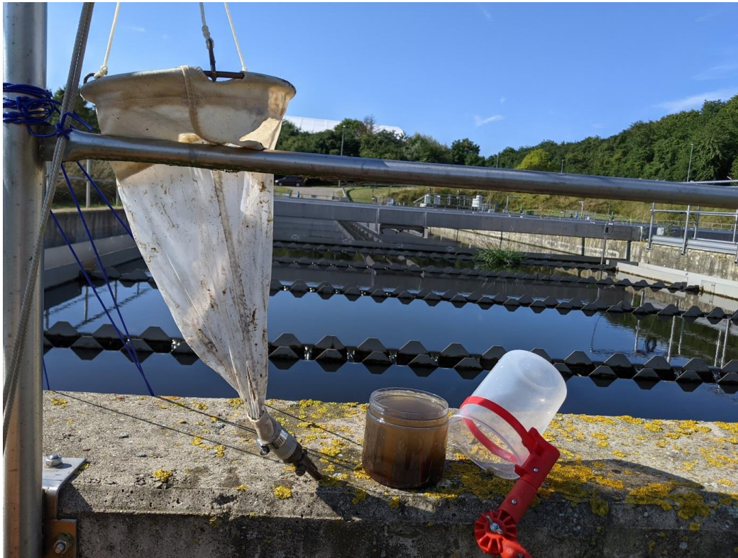
Figure S1. The zooplankton sampling net for sampling of Daphnia sp. from clarifiers (at back of picture)
