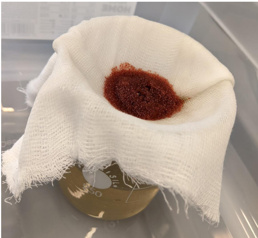
Figure S2. The separation of daphnia organism from water and particles using medical gauze
