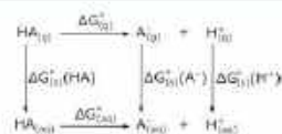
Figure 3. Thermodynamic cycle used 23 for the calculation of pK_{a,calc} according to the direct method. The g superscript denotes the condition of 1 atm, whereas the aq represents 1 M.
