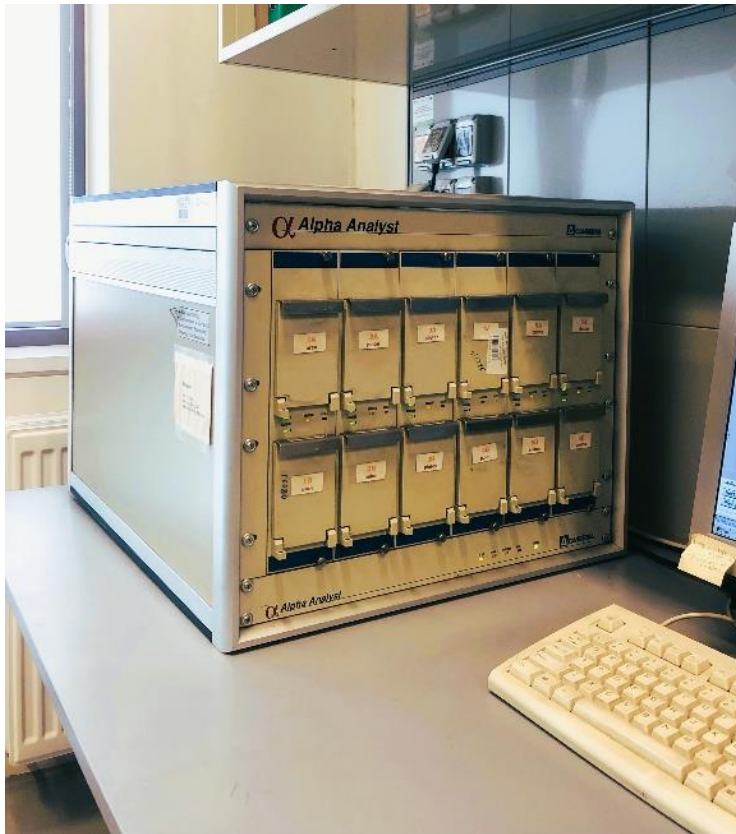
Figure 25. Alpha spectrometer at the University of Gdańsk
