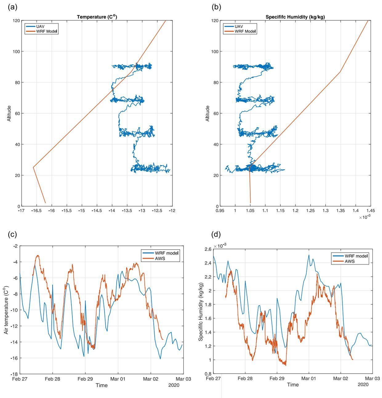
Figure 2 Measured (HAOS UAV) and modeled (WRF) vertical air properties off the coast of Hailuoto Marjaniemi on the 1st of March 2020, (a) temperature (b) specific humidity, and AWS measurements and WRF model results for the period of HAOS campaign (27 February- 2 March 2020) of (c) air temperature and (d) specific humidity 2 m above the surface.
